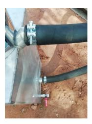
With the taps you can control the circulation of the water so that the water flows faster and / or slower to regulate the temperature of your water. In the beginning, set 1 of the 2 taps to a quarter and as the water gets warmer, slowly turn it on until it is fully open.
