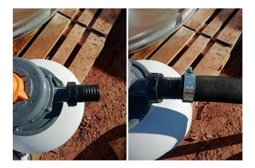
Do not forget to put the supplied sealing rings in order to prevent water leakage to the connections. Use Teflon if needed to avoid leaks. Slide the hose clamps over the two heat hoses provided at each end.
