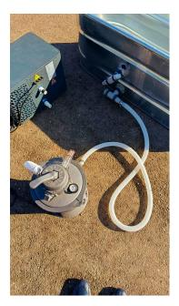
Connect the lowest inlet on the tank with the lowest inlet on the filter pump. Use the clamps to tighten.
