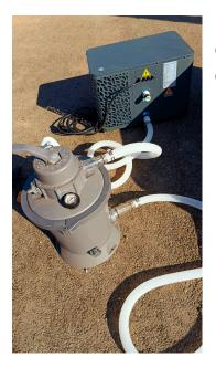
Connect the highest inlet on the filter pump with lowest inlet on the chiller/heater. Use the clamps to tighten.
