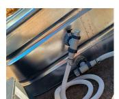
Connect the highest inlet on the chiller/heater with the highest inlet on the tank. Use the clamps to tighten.
