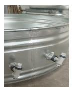
This is a picture from the outside of the tank. Both inlets with the valves connected, ready to connect the hoses with clamps.
