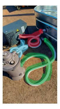
When you've connected everything and when you tighten all the rings around the hoses, switch the valve on the sandfilter pump to 'filtration' and open the 2 valves on your pool (connected on the inlets).
